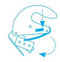
Press the catch and remove the metal foot from the handle. Replace or reverse the blade.
