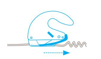
Whether cutting foam or film, the bendable plastic material-guide reliably stops material jamming in front of the blade.
