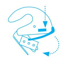
Press the catch and remove the metal foot from the handle. Replace or reverse the blade.
