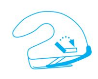
**Lift** the catch and move downwards until its end covers the blade change button.
