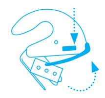
Press the catch again and insert the metal Move foot back into the handle until it **clicks**. Check **tion**. that the foot is correctly inserted.
