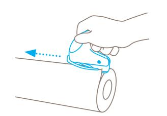
**Pierce** film and paper sheets at the required position using the point of the metal foot.
