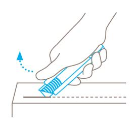
Remove your **thumb from the slider** to ensure automatic blade retraction.
