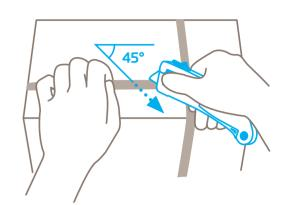
For best results, cut plastic strapping band **diagonally** (at a 45° angle).
