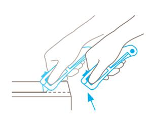
The blade automatically retracts into the handle the moment cutting ceases. Even when the slider is still **being held forwards**.
