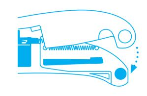
Finally, fold the **upper half of the handle back down** until it snaps into place. Please check blade retraction!
