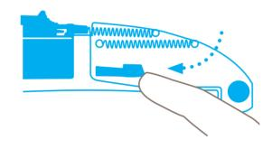
Release the blade carrier by **pressing down** and pushing forward, as indicated.
