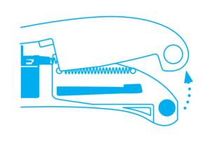
To change the blade, **press the button** at the end of the knife and fold open the upper half of the handle.
